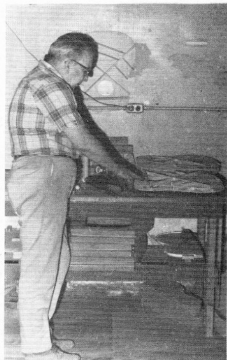
Checking the strength of the spruce tops, Mr. Gallagher notes that this is one of the most important steps in construction.
