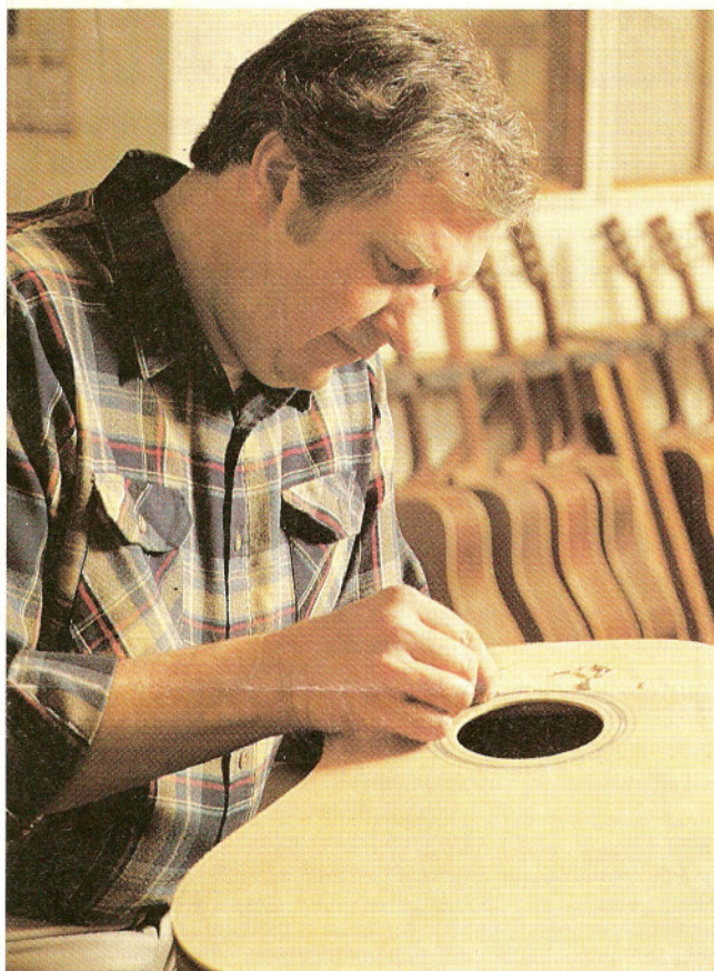
Tennessee's Don Gallagher carefully places pearl inlay around the sound hole in one of his guitars, which he makes by hand.
